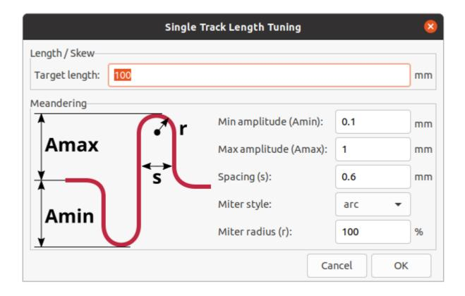
This dialog can also be used to configure the size, shape, and spacing of the meander shapes.
