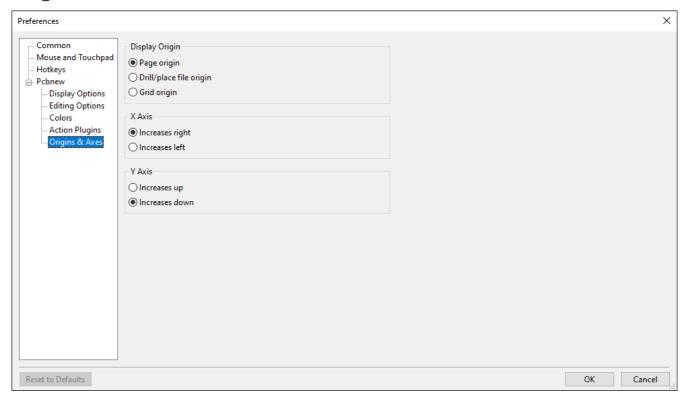
**Display origin:** Determines which coordinate origin is used for coordinate display in the editing canvas. The page origin is fixed at the corner of the page. The drill/place file origin and the grid origin can be moved by the user.
