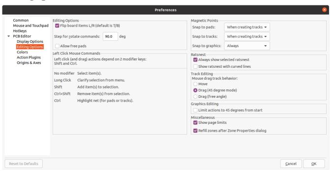
Flip board items L/R: Controls the direction board items will be flipped when moving them between the top and bottom layers. When checked, items are flipped Left-to-Right (about the Vertical axis); when
