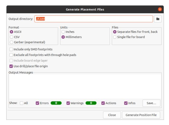
**Format:** Choose between generating a plain text (ASCII), comma-separated text (CSV), or Gerber placement file format.
